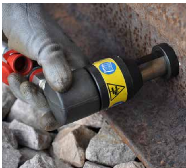
RHTEP while extruding AR contact
